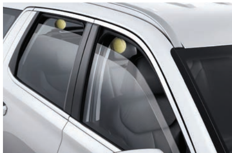
Power window with anti pinch
